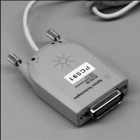
**Fig 7: A USB GPIB adaptor (Agilent 82357B).**
